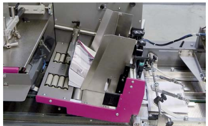
W+D HF2 hybrid – friction/vacuum feeder
