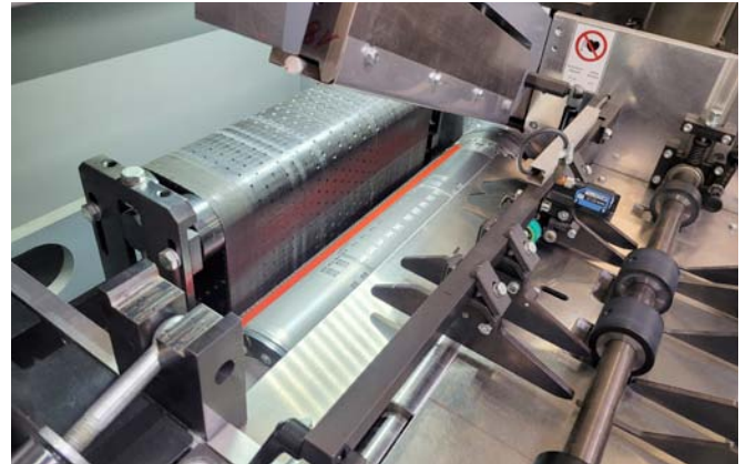
Complete cut using foil knife on magnetic cylinder, vertical vacuum transport
