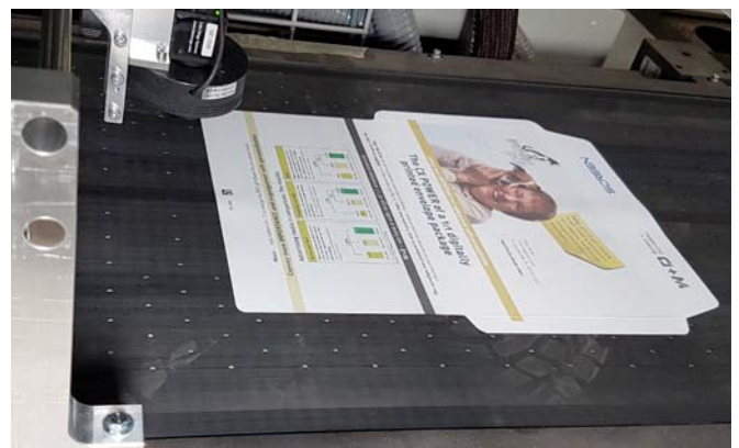
A camera capturing the 2D code on the lead edge of the envelope blank
